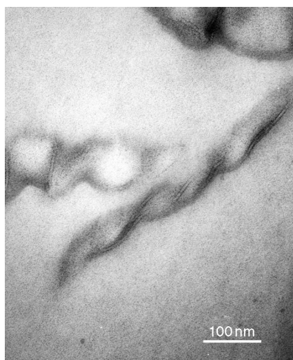
Figure 5.56 Transmission electron microscope bright field image of a twisted single lamella of ultrahigh molecular weight polyethylene in a decalin solution. Decalin was replaced by methacrylate that was polymerized to yield crystals of the polyethylene crystal embedded in a solid poly (methacrylate) matrix, while its original morphology was retained. The sample was microtomed and stained with ruthenium tetroxide [reprinted from Kunz et al. (1995), with permission].
